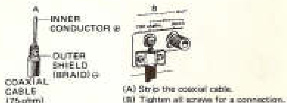
Fig. 4 — Connect coaxial cable to 75Ω UNBAL.
